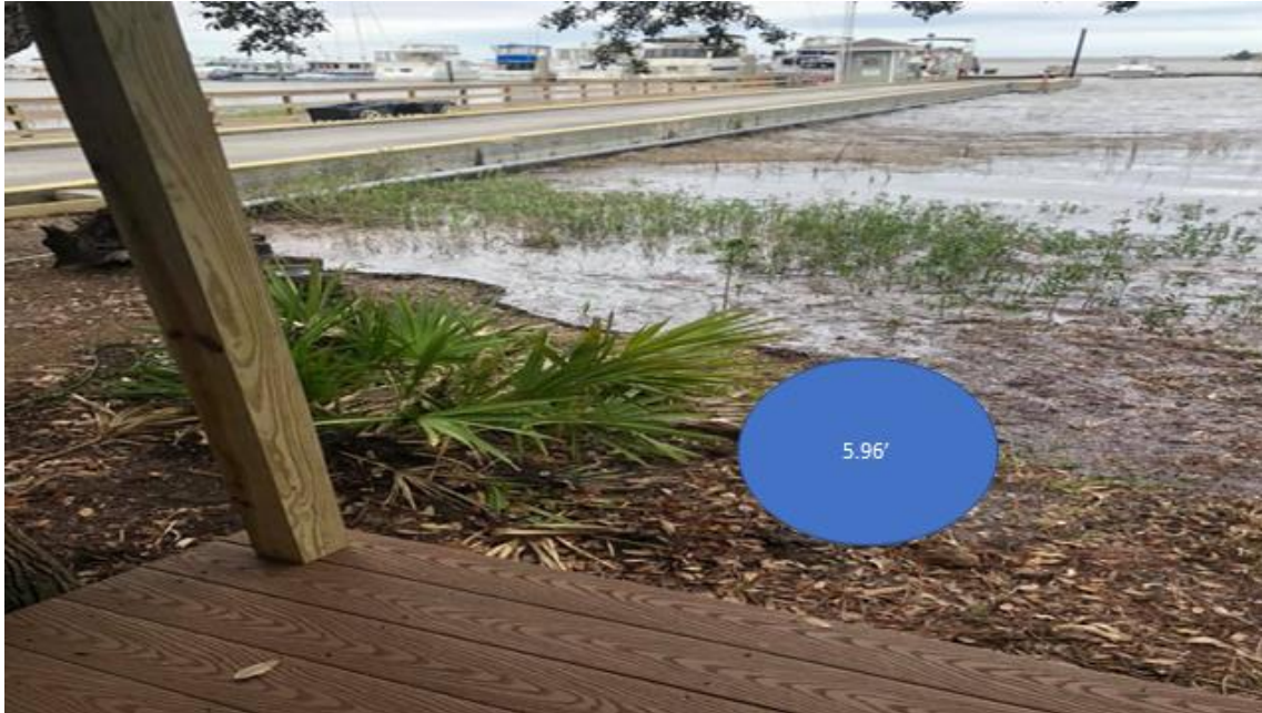
Figure 1. This photo taken on February 19, 2019 shows the level of tide-water during a spring tide event in conjunction northeasterly wind flow. The water level elevation is estimated at 5.96' (NAVD88 datum – comparable to Mean Sea Level (MSL)) .
